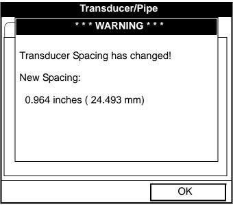
Figure 14: Transducer Spacing Change Window
